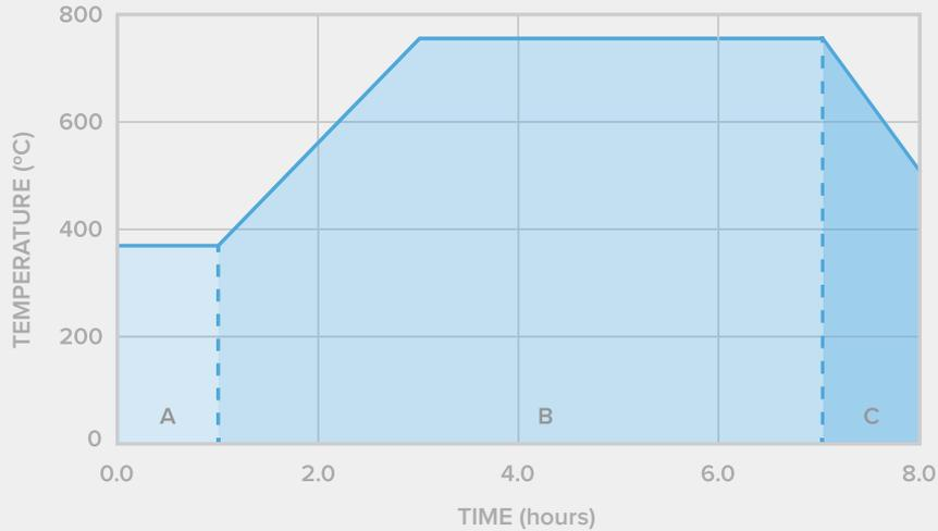
It is possible to achieve faster cycle times with some geometries and investment materials. Higher end investments, such as R&R's Ultravest Maxx, are stronger and can withstand faster heating.
