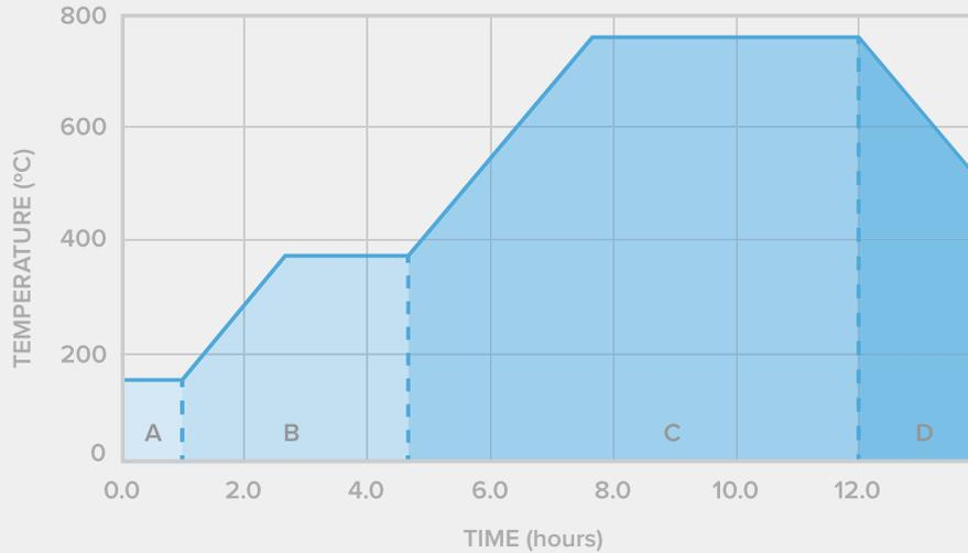
The Standard Burnout Schedule is designed to provide the maximum possible investment strength and complete burnout of the finest details using R&R Plasticast or similar investment materials. Use this schedule as a starting point and make adjustments as needed.
